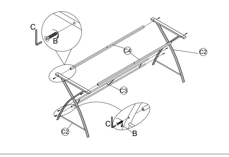
STEP 2: Use Hex Key(C)to tighten the Top panel(C1) to Connect bar(C4) and Legs (C2)with Bolt (A)
